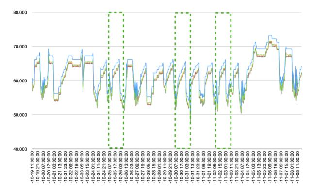
Overview of sample monitors and reference Airsns NANO temperature(blue) readings. Peaks from the following tables are taken from the maxima in the green boxes.
