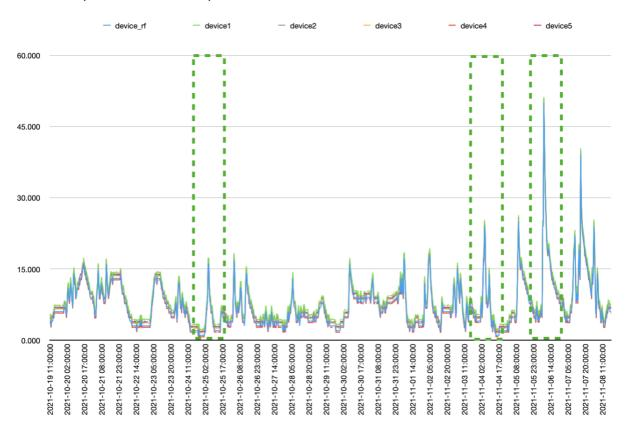
Overview of sample monitors and reference Airsns NANO PM2.5(blue) readings. Peaks from the following tables are taken from the maxima in the green boxes.
