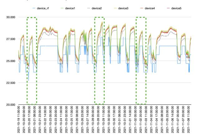
Overview of sample monitors and reference Airsns NANO temperature(blue) readings. Peaks from the following tables are taken from the maxima in the green boxes.
