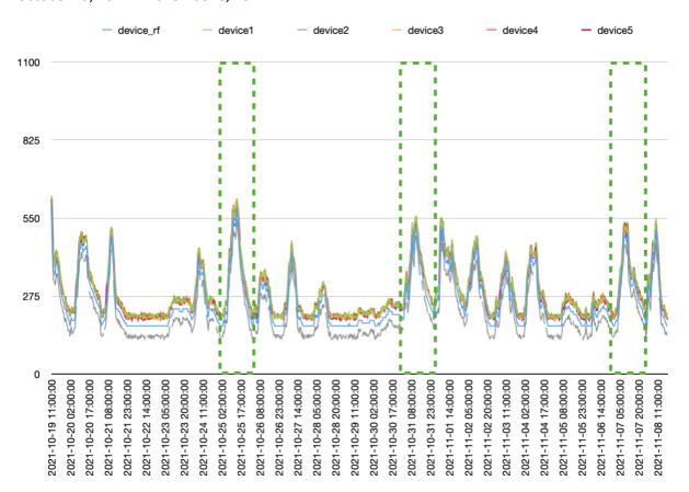
Overview of sample monitors and reference Airsns NANO TVOC(blue) readings. Peaks from the following tables are taken from the maxima in the green boxes.
