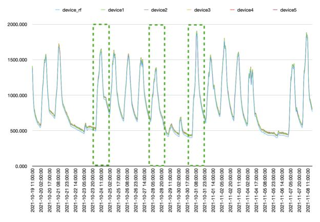
Overview of sample monitors and reference Airsns NANO CO<sub>2</sub> (blue) readings. Peaks from the following tables are taken from the maxima in the green boxes.
