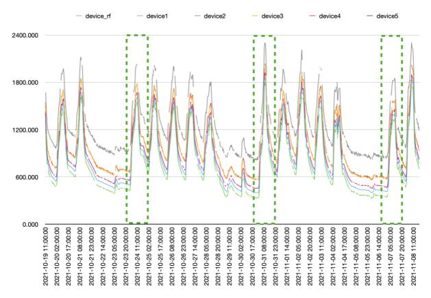
Overview of sample monitors and reference Airsns NANO  $CO_2$  (blue) readings. Peaks from the following tables are taken from the maxima in the green boxes.
