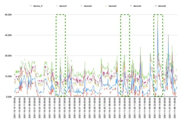
Overview of sample monitors and reference Airsns NANO PM2.5(blue) readings. Peaks from the following tables are taken from the maxima in the green boxes.
